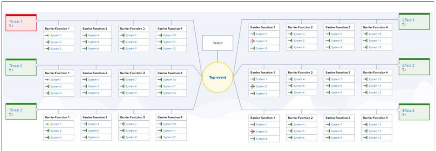
Synergi Life Barrier Management - Full bow tie diagram with integrity levels and relevant connections.
