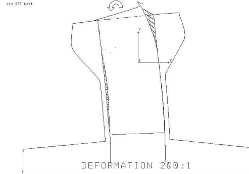
Fig. 2 FE Analysis Model of the foundations at Middelgrunden showing the deformed shape from the FE analysis calculations.
