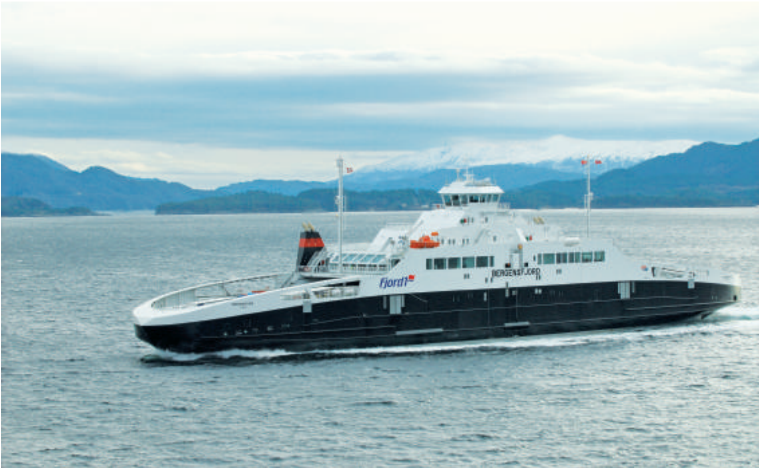
The exhaust emitted from the LNG-powered car ferry "Fanafjord" (front cover) is rather clean. "Fanafjord", as well as its sister ship "Bergensfjord" (above), has virtually no SOx or NOx emissions and the CO 2 is substantially below a conventional diesel powered ferry. The future solutions for low carbon shipping are already available.
