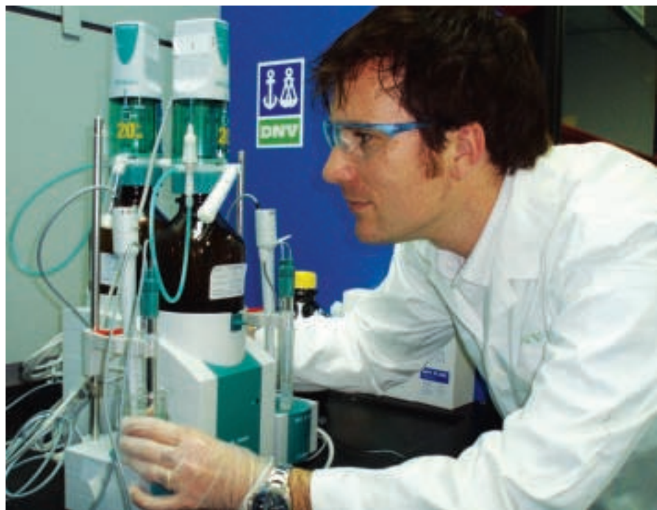
DNV Petroleum Services lab analyst running Base Number analysis on cylinder lubricating oil.
